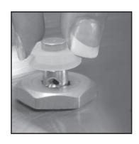
4. The Float Valve should be able to move up and down freely only stopping when the silicon gasket meets the Lid.
