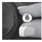
Hold the head of the Float Valve and insert the fluted end into the hole in the Lid of the unit with a pencil or any other slim tool. Push and hold the head of the Float Valve tightly in place and reverse the Lid to the underside.
