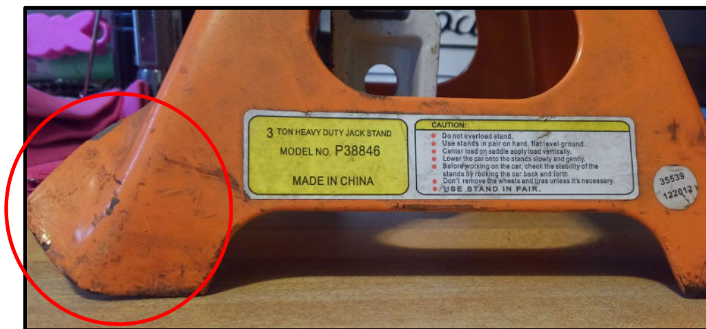
Subject jack stand labeling and leg deformation
