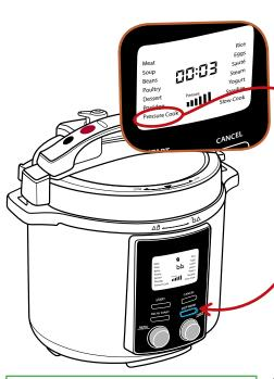
NOTE: For the duration of time the unit is cooking with pressure, and until the pressure is released, the Float Valve will be raised and the lid is locked. NEVER ATTEMPT TO OPEN THE LID FOR THE DURATION OF THE PRESSURE COOKING TIME.
